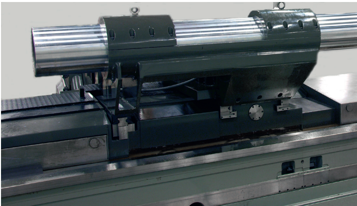
Split holder for 300 mm (11.81 inch) bar diameter. The distance between the cross slides is 1,200 mm (47.24 inch) (4 x BD).
